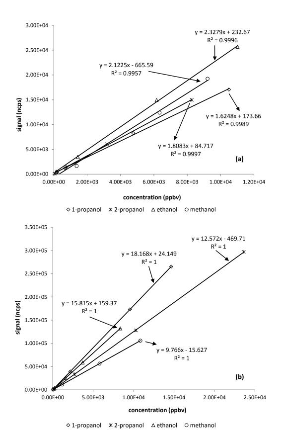
**Figure 1.** Calibration curves for 1-propanol, 2-propanol, ethanol and methanol at physiologically representative concentrations; data acquired using SIFT-MS (a) and PTR-MS (b).
