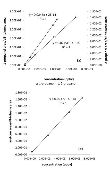
**Figure 4.** Calibration functions using the internal standard procedure for 1-propanol, 2-propanol (a) and acetone (b); data acquired using TD-GC-MS.
