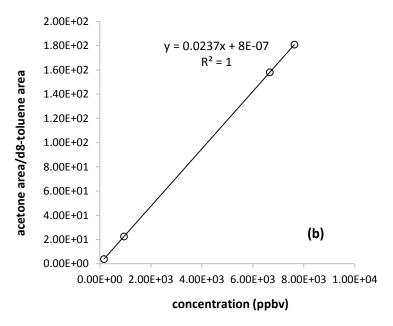
**Figure 5.** Calibration functions using the internal standard procedure for 1-propanol and 2-propanol within a mixture of VOCs (a) and acetone (b); data acquired using TD-GC-MS.
