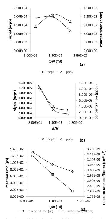
**Figure 3.** (a) Concentration of acetaldehyde in ppbv and (b) 2-propanol in ppbv, calibrated to 5 ppm in the gas-phase, and normalised counts per second (ncps) as a function of reduced electric field strength (E/N = 90, 125, 160); (c) Acetaldehyde- $H_3O^+$  reaction time and reaction rate coefficient as a function of E/N = 90, 125, 160.
