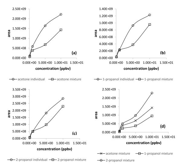
**Figure 6.** Comparison of the peaks areas observed in chromatograms acquired using TD-GC-MS for individual calibration solutions, and peak areas acquired for a VOC mixture containing the six VOCs analysed (a) acetone, (b) 1-propanol, and (c) 2-propanol; (d) comparison of peak areas within the VOC mixtures at gas-phase concentrations of 0.1 ppm, 1 ppm, 5ppm, and 10 ppm.
