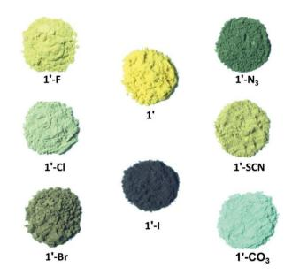
**Figure 1.19.** Images showing the colour change in MOF Cu(pytpy)](NO<sub>3</sub>)·(CH<sub>3</sub>OH) as result of anion-exchange. Reproduced from reference 16.
