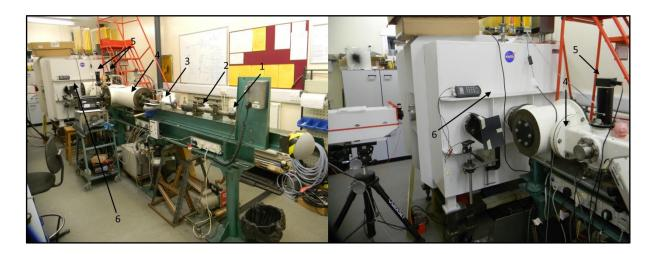
Figure 1 - Labelled images of the Light Gas Gun showing its major components: (1) Powder Chamber, (2) Pump Tube, (3) Launch Tube, (4) Blast Tank, (5) Dual Laser Blanket connected to oscilloscope, (6) Target Chamber.
