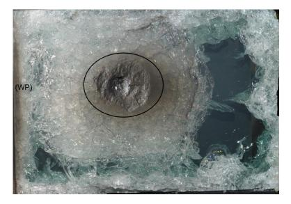
Figure 32 - Photo showing the extent of the glass block shattering post hypervelocity impact. As before, (WP) shows the witness plate end of the target, and the impact crater is bounded by the black ring.
