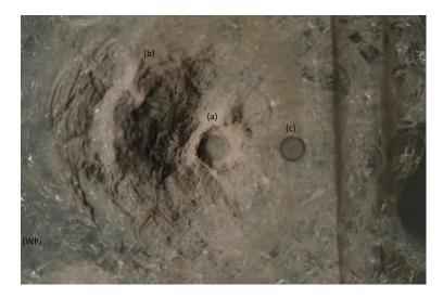
Figure 40 - Image showing the impact crater in the soda lime glass target, where (WP) shows the end of the glass block were the witness plate is fixed, (a) is the crater pit, (b) is the area of dislodged material from the glass block, and (c) is the 2.5mm size marker.
