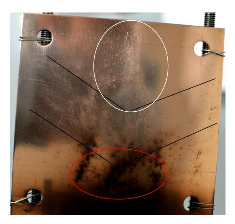
Figure 41 - Image displaying the secondary ejecta pattern on the copper witness plate. The black chevron indicates the previously seen fan pattern, the red ellipse shows the area below the fan centre made up of trailing marks, and the white ellipse bounds the now better-defined 'peak' pattern.
