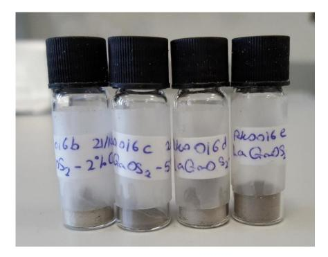
Figure 5.14 Colour change in each of the different Ce doping concentrations form the initial pale-yellow colour after reaction.  $La_{0.98}Ce_{0.02}GaOS_2$  (far left) became pale-grey,  $La_{0.95}Ce_{0.05}GaOS_2$  (second from the left) became grey,  $La_{0.93}Ce_{0.07}GaOS_2$  (third from the left) became pale-grey and  $La_{0.9}Ce_{0.1}GaOS_2$  (far right) became grey.
