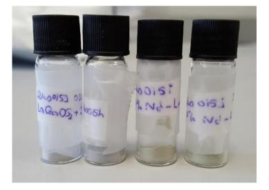
Figure 5.08 Colour change in each of the different Nd doping concentrations form the initial blue-green colour after reaction.  $La_{0.98}Nd_{0.02}GaOS_2$  (far left) became pale-grey,  $La_{0.95}Nd_{0.05}GaOS_2$  (second from the left) became pale-grey,  $La_{0.93}Nd_{0.07}GaOS_2$  (third from the left) became green-grey and  $La_{0.9}Nd_{0.1}GaOS_2$  (far right) became apple-green.
