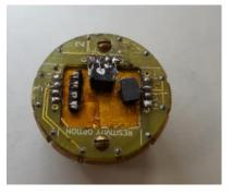
Figure 2.14 Puck with samples ready for electrical resistivity measurements
