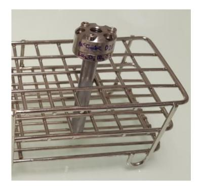
Figure 2.08 Sample in vanadium can ready for neutron diffraction measurements
