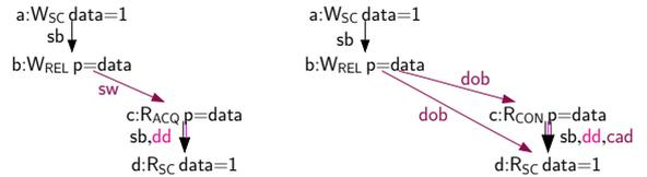
For release/consume, the key fact is that there is a *data dependency* (dd) from (c) to (d), as shown on the right. The (dd) edge is provided by the operational semantics and gives rise to a *carries-a-dependency-to* (cad) edge, which extends data dependency with thread-local reads-from relationships:
