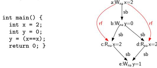
The set of actions and the sequenced-before relation are given by the operational semantics (so are part of the  $X_{\text{Opsem}}$ ); the *rf* relation is existentially quantified (part of the  $X_{\text{witness}}$ ), as in general there may be many writes that each read might read from.
