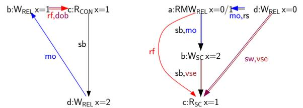
The execution on the left violates CoRW by containing a cycle of happens-before and modification order edges, allowed only due to the lack of transitivity of happens-before. The execution on the right violates CoWR by having a read from a write (the read-modify-write (a)) that is sequenced-before-hidden by (c). Actions (b) and (c) are shown as SC atomics for emphasis.
