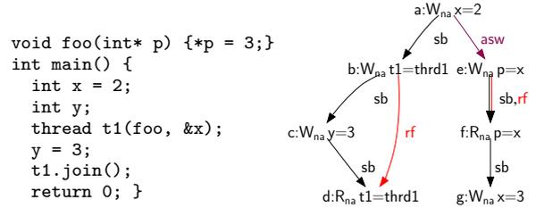
The thread creation gives rise to *additional-synchronizes-with* (asw) edges (here  $a \xrightarrow{\text{asw}} e$ ) from sequenced-before-maximal actions of the parent thread before the thread creation to sequenced-before-minimal edges of the child. As we shall see, these edges are also incorporated, indirectly, into happens-before. They are generated by the operational semantics, so are another component of an  $X_{\text{Opsem}}$ .
