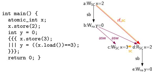
Semantically, this is because SC atomic operations are totally ordered by  $sc$ , and so can be thought of as interleaving with each other in a global time-line. Their semantics are covered in detail in [BA08] and we will describe their precise integration into happens-before in the following section.
