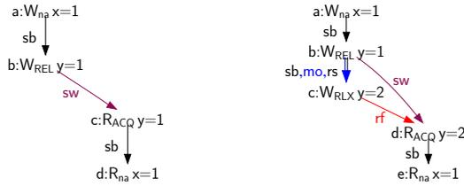
For such programs (in fact for any program without release/consume atomics), happens-before is still the transitive closure of the union of the sequenced-before and synchronizes-with relations, so here  $a \xrightarrow{\text{happens-before}} d$  and (d) is obliged to read from (a).
