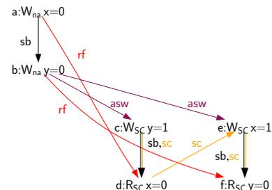
We devised a stronger restriction on the values that may be read by SC atomics, stated in §2.7, that does provide sequential consistency here.
